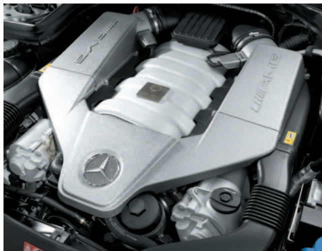
M156 V8 with bore and stroke of 102.2x94.6mm plus two cams per bank; max power arrives at 6,800rpm.
